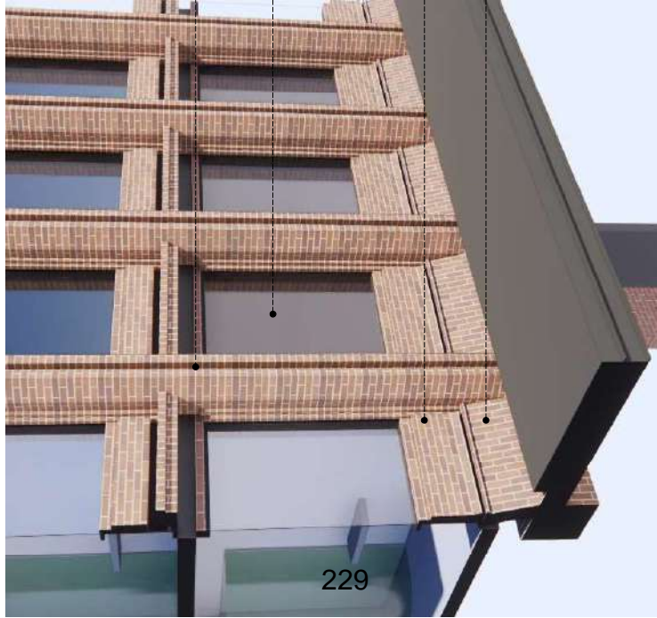
1 PODIUM FACADE DETAIL - LEVEL 01
