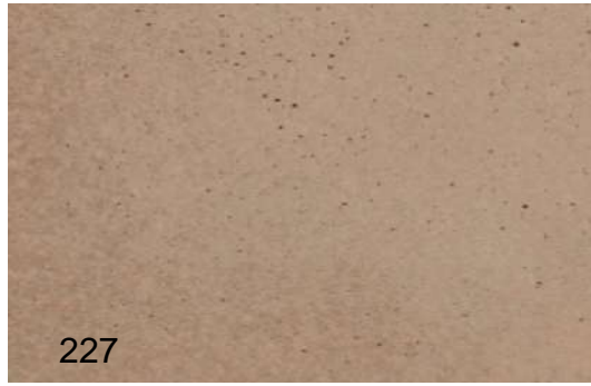
PC01 - COLOURED PRECAST PANELS TO MATCH BRICK - FOR WALL A01
